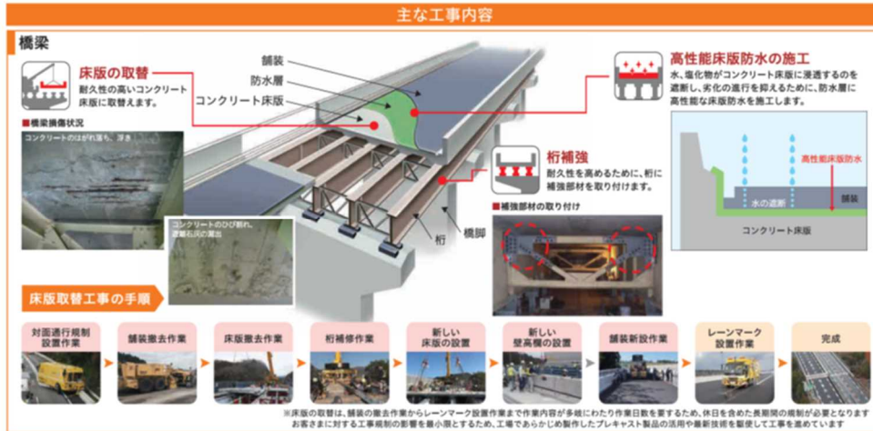
Figure 3: Detailed Construction on Bridge Slabs 6
